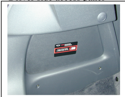
Driver side access panel
